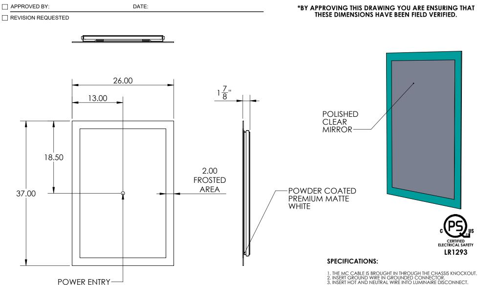
3. INSERT HOT AND NEUTRAL WIRE INTO LUMINAIRE DISCONNECT.
